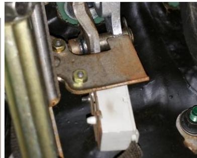
Shown is the Neutral Start Switch removed and the mounting bracket from under the dash.
